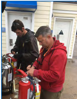
Fire extinguishers being serviced.
